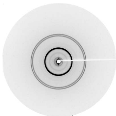
Fig. 7 X-Ray pattern in the low-angle region of a non-oriented D9F23 sample: several reflections are seen ( q = 0.048 \text{ \AA}^{-1} , 0.158 \text{ \AA}^{-1} , 0.302 \text{ \AA}^{-1} , 0.322 \text{ \AA}^{-1} ) but the structure cannot be determined without an oriented sample. Note that, increasing the chain length, the weaker reflections vanish and as for a smectic phase, an intense reflection with its first harmonic only is detected.
